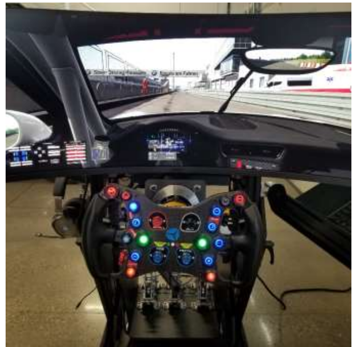
SIM cockpit from the driver's seat. Pedals below, screen above with dash and instrument display, track ahead.
