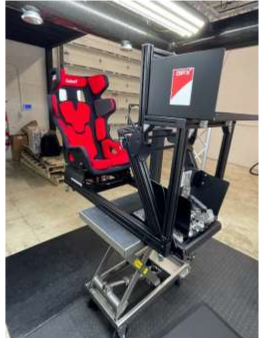
The bare SIM platform before all the electronics are installed.
